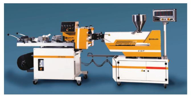
Testing extruder 30 mm diam. type E 30 P, slot die 250 mm and finishing calender type 136/350
