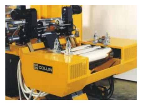
Edge cutting with motor-driven circular blades.
