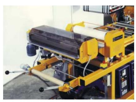
Take off with winder for film or traversing saw for cutting sheet.
