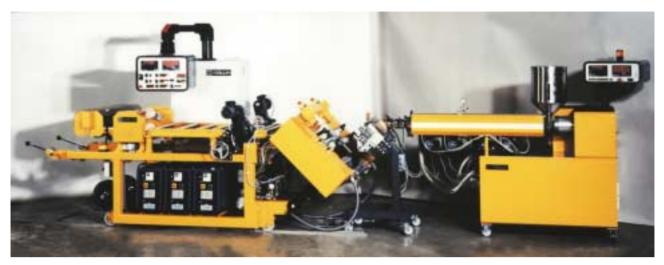
Laboratory sheet line with extruder, 45 mm diam. x 25 D, slot die 450 mm on a mobile frame, roll unit in 45° position, motor-driven edge cutting unit, take-off rolls, traversing saw, film winder, edge-strip winder and integrated hot water temperature control units.
