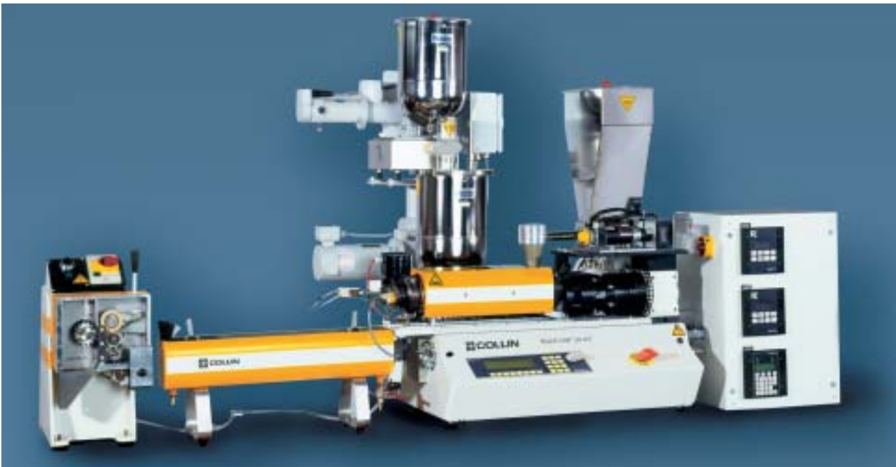
Compounder ZK 25 T x 18 D with Waterbath WB 850 T and Pelletizer CSG 171 T; volumetric feeding for the main feeding part, gravimetric feeding for the side-feeder.
