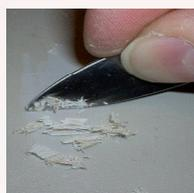
With this technology combination practically all common types of plastics, regardless of color, size, structure (films, foils, granules, solid, foamed, carpets and textiles) can be identified together with their additive elements like fire retardants and heavy metals. For sample preparation to remove dust and dirt or paintings the sample surface can be easily cleaned by scratching with a knife.
