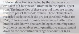
The identification of PVC is possible by high concentrations of Chlorine measured.
