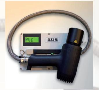
The portable sliding spark spectrometer allows the following samples to be analyzed within 1 second and independently of colour:
