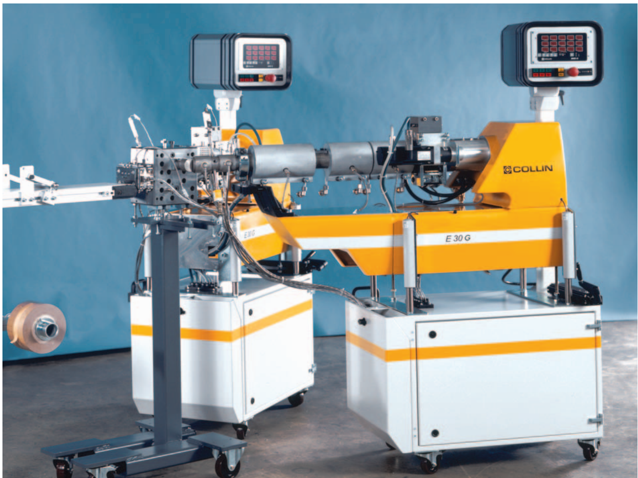
Line for the production of multi-layer flat profiles
