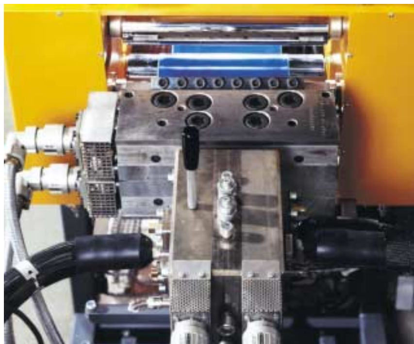
Section through a 5-layer feedblock for the production of symmetrical or asymmetrical layered materials.
