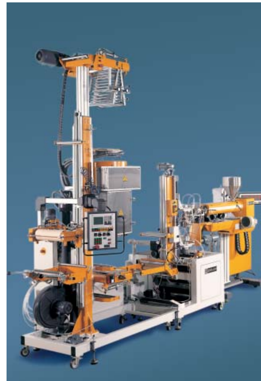
3-layer coextrusion line for film with water cooling of the primary film and IR-heating zone for biaxial stretching of the secondary film
