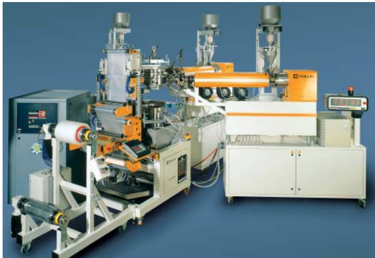
3-layer quenching line for the production of infusion bags
