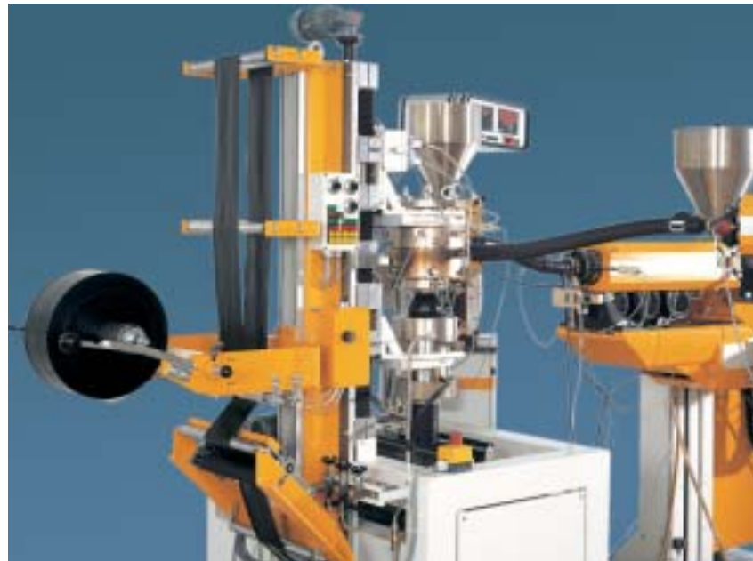
3-layer blown film line with water cooling for the production of tubes with small diameters
