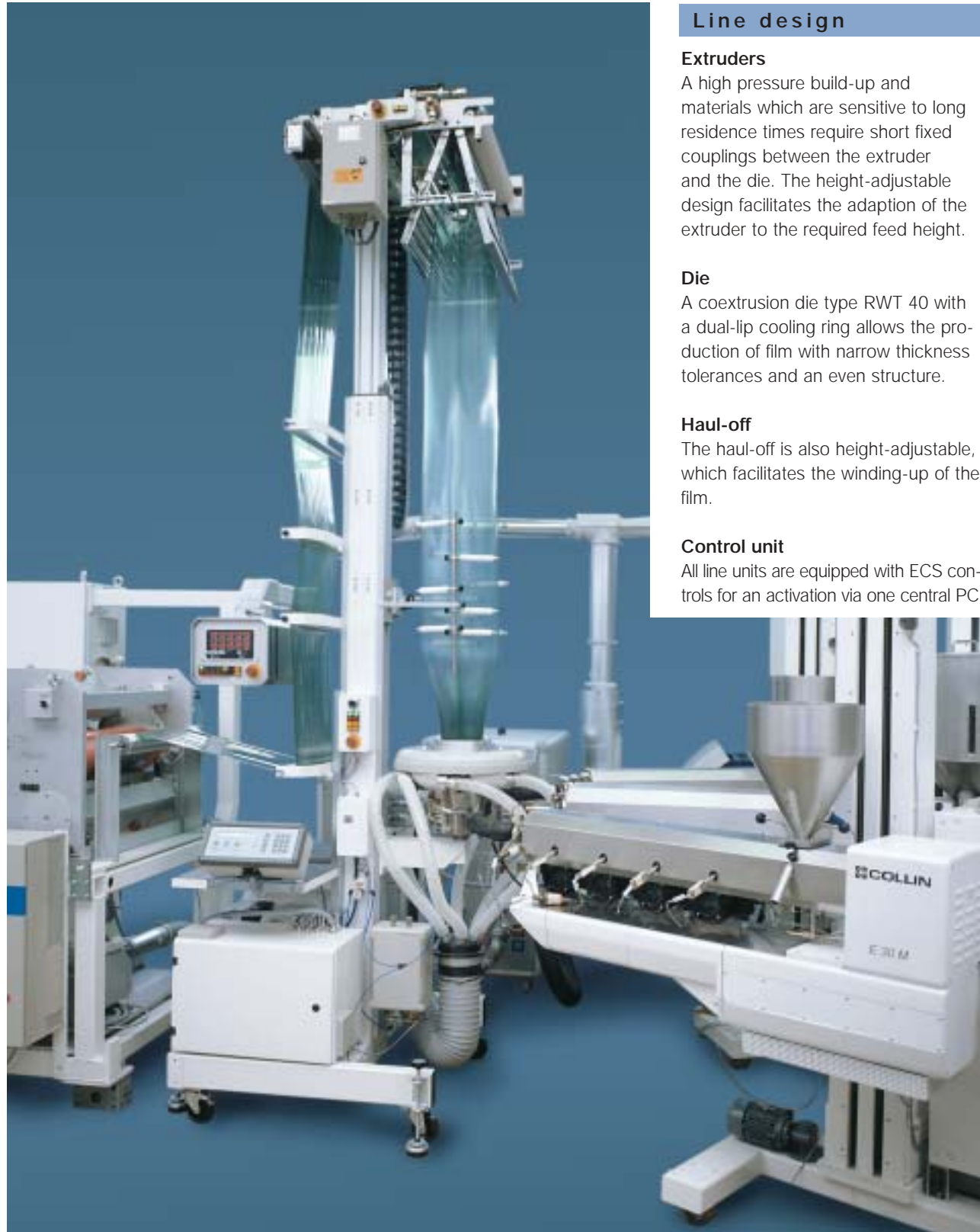
3-layer blown film line with 3 extruders 30 mm, 30 mm and 45 mm diameter extruders
